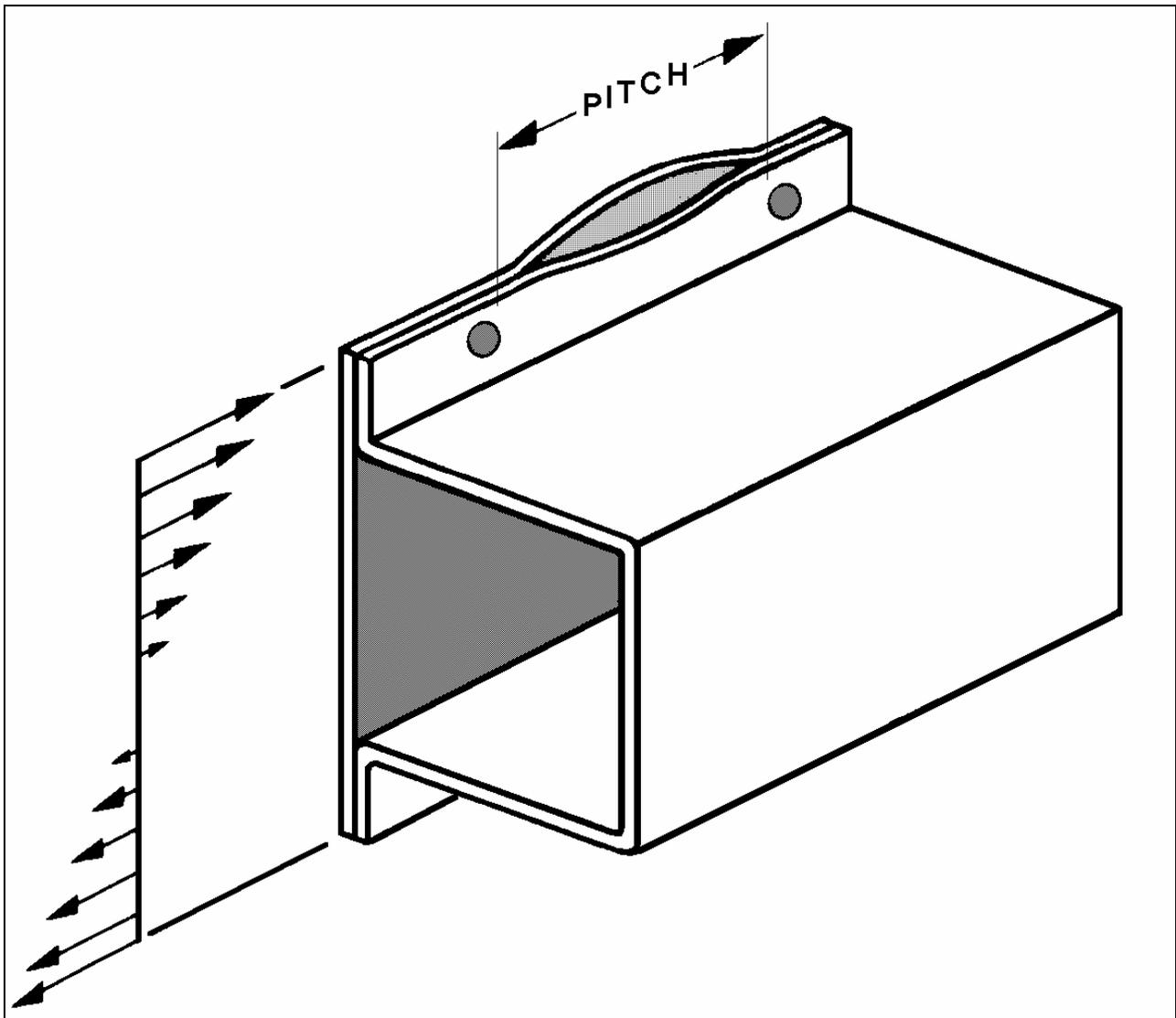
*Figure 6: Flange gap in spot welded Hat sections with cover plate under bending*
