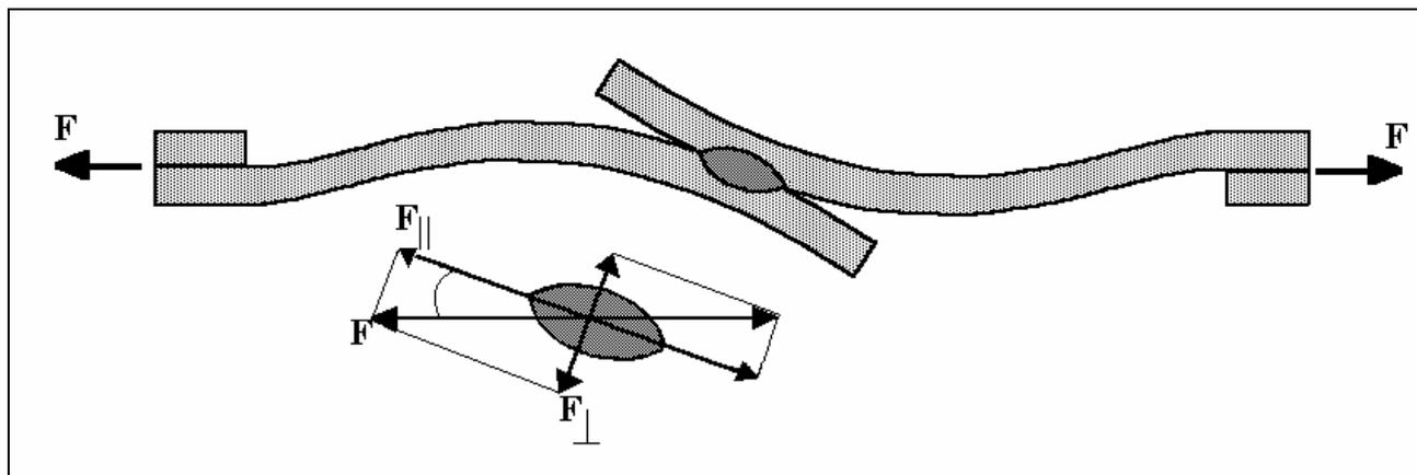
*Figure 5: Slanting of weld spot subjected to tensile shear, superimposed cross tension by slanting*
