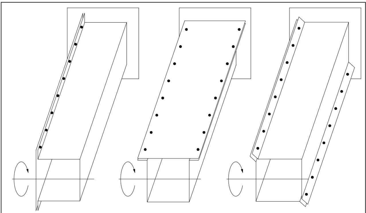
*Figure 7: Three different spot welded hat section arrangements*
