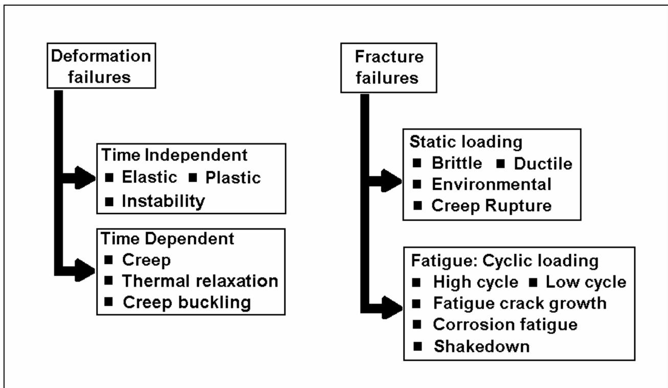
*Figure 1: Basic Types of deformation and fracture failures*
