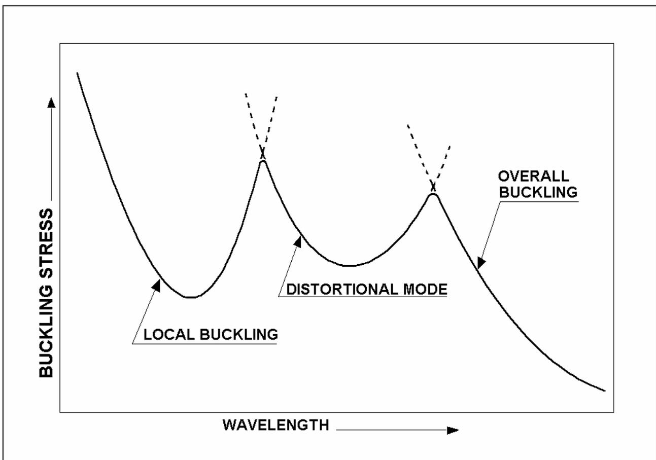
*Figure 2: Evaluation of the buckling stress*
